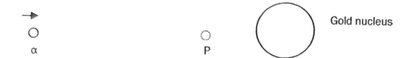
Point P is the closest point that the  $\alpha$ -particle can get to the nucleus before being repelled. At point P the KE of the  $\alpha$ -particle is zero as it stops momentarily. All of its energy has now been converted into PE.
