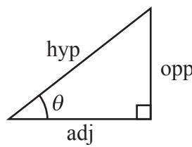
$$\begin{aligned}\text{adj} &= \text{hyp} \times \cos \theta \\ \text{opp} &= \text{hyp} \times \sin \theta \\ \text{opp} &= \text{adj} \times \tan \theta\end{aligned}$$
