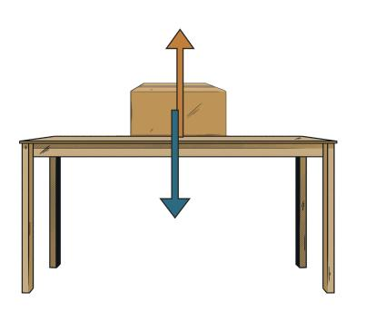
The upwards arrow represents the **reaction** force. This is the force of the table supporting the box.
