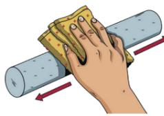
When a polythene strip is rubbed with a cloth, electrons move from the cloth to the strip. The strip becomes negatively charged and the cloth becomes positively charged.
